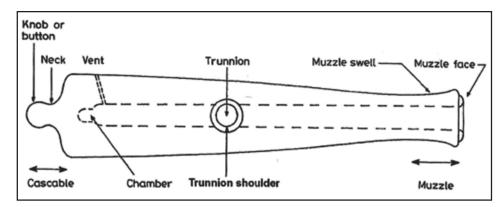
Fig.1. Schematic diagram showing the various parts of typical cannon
