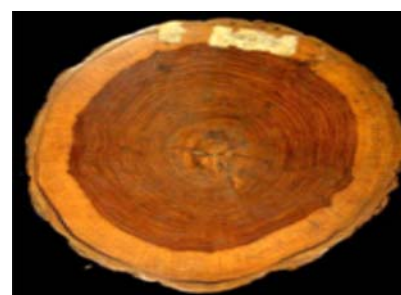
Fig. 70. A transverse section of the log showing prominent heartwood in the centre and sapwood in the periphery
