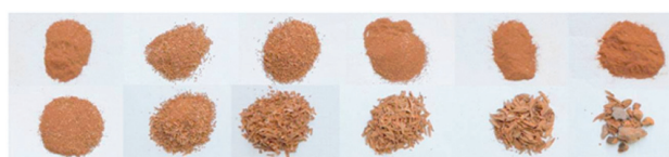
Fig. 6. Aggregates in mud plaster of Bhaja caves.
