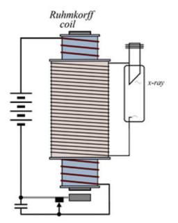
Fig. 5. Schematic diagram of X-ray apparatus using a Ruhmkorff's coil as a high voltage source as was used by Roentgen.
