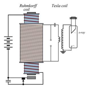
Fig. 6. Schematic diagram of Tesla coil coupled with Ruhmkorff's coil, the apparatus which Jagadis Chandra probably used as a high voltage source to the X-ray tube
