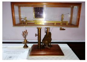
**Fig. 2.** Compound Lever Crescograph– An apparatus invented by JC Bose in early 20<sup>th</sup> century, on display at the Bose Museum in Kolkata.
