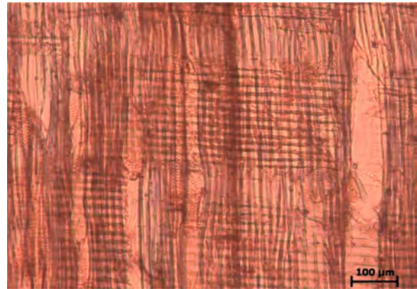
Figure 11 R.L.S. of Populus sp. showing homogenous rays at 100x.
