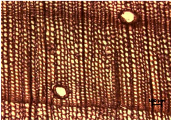
Figure 19 T.S. of Pinus wallichiana showing growth ring and canal at 50x.
