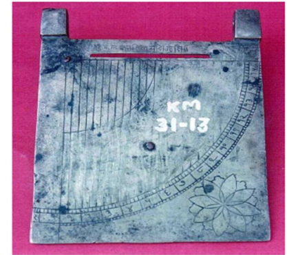
Figure 2: Dhruvabrahma-yantra , made for Yado Joshi, resident of Ukala-grāma (Akola), latitude 20 degrees. Reverse side, with the sine quadrant. Raja Dinkar Kelkar Museum, Pune.
