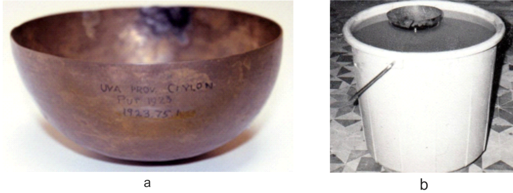
Figure 1 (a) Copper bowl water clock sinking in half ghaṭi from Uva Province, Sri Lanka in the Pitt Rivers Museum of Ethnology, Oxford. (photo by S. R. Sarma); (b) Coconut shell water clock sinking in one ghaṭi . Government Museum, Chennai. (photo by S. Ramaratnam)
